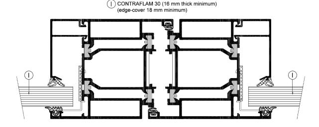
The doorset shall have test evidence or be CERTIFIRE approved for the inclusion of apertures of the proposed dimensions. This Certificate of Approval relates to the sizes of Contraflam 30 glass shown in the table below, when used in conjunction with the above system:
