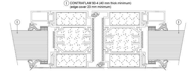
The doorset shall have test evidence or be CERTIFIRE approved for the inclusion of apertures of the proposed dimensions. This Certificate of Approval relates to the sizes of Contraflam 90-4 glass shown in the table below, when used in conjunction with the above system:
