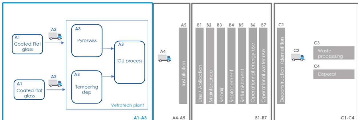
Figure 1 : Relevant LCA steps for VETROFLAM IGU Steps in blue are declared in this EPD, steps in grey are not declared.
