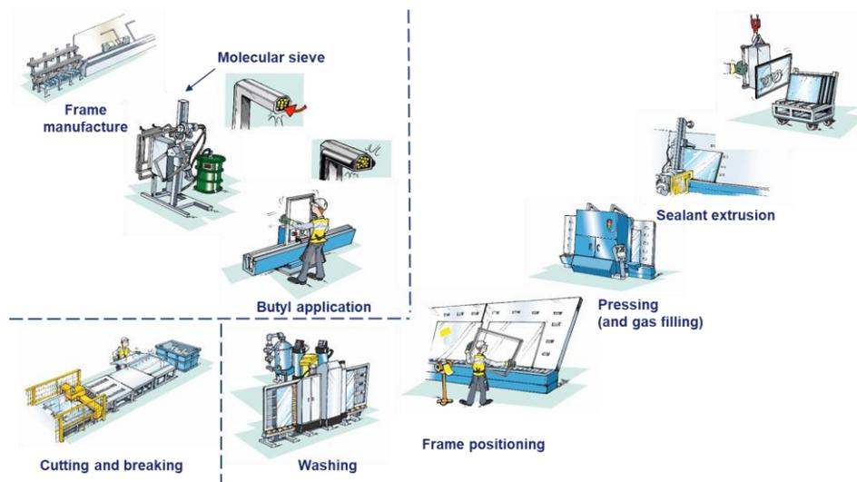
1. **GLASS PREPARATION:** Glass plates are cut to be at the good dimension for the final product. Glasses are cleaned and dried.
