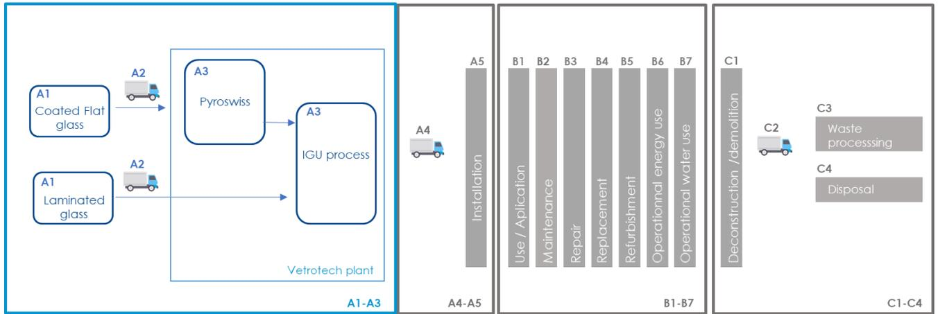
Figure 2 : Relevant LCA steps for VETROFLAM IGU with laminated glass. Steps in blue are declared in this EPD, steps in grey are not declared.
